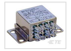
Type of Control: Fixed Time Delay Relay Input Voltage: 28 VDC Time Delay Relay Contact Current Rating: 10A@28VDC A, 115VAC A Mode of Operation: Delay on Operate Delay Time: **30 seconds**
